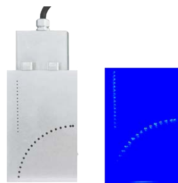
ASME steel block inspection, using 5 MHz LO° phased-array probe with 64 elements
